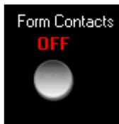
Press the Form Contacts button to run a sample contact formation algorithm. Initially, a setup screen will be displayed allowing the user to input parameters that control the algorithm. This button cannot be pressed when a experiment or profile is being executed.
