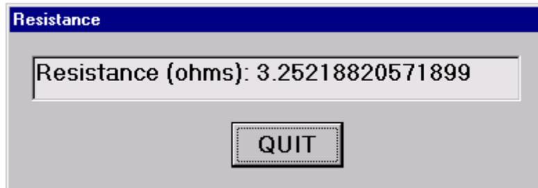
This window displays the current resistance and updates the resistance twice a second. If the sourcemeter is in voltage compliance, a compliance message will be displayed instead of the resistance.
