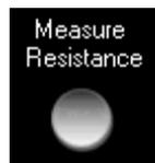
Press the Measure Resistance button to get the resistance of the sample. Initially, a setup screen will be displayed allowing the user to input parameters that control the measurement. This button cannot be pressed when a experiment or profile is being executed.
